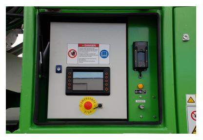
Unloaders with these advanced PLC systems have almost unlimited troubleshooting potential, both on site and remotely, including the ability to conduct self-diagnostic system runs and software upgrades directly from Bruks Siwertell. The fieldbus system also allows for a significant reduction in cabling, in comparison to older models, throughout the equipment.
